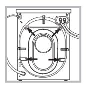
3. Remove the four protective screws and the rubber washer with the respective spacer, situated on the rear of the appliance (see figure).
